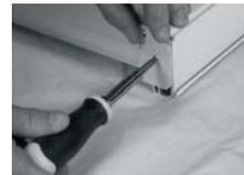
Install the cord tensioner by unwinding the cord from the end plate. Slide the cord tensioner into the channel at the front of the headrail.
