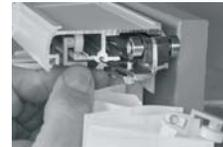
Install the cord tensioner by unwinding the cord from the end plate. Slide the cord tensioner into the channel at the front of the headrail.
