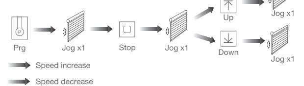
Note: If motor doesn't jog, the max/min speed has already been reached. There are 3 adjustable speeds.
