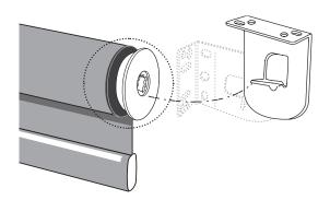
**B** – The idler end has a spring-loaded pin that allows it to compress in/out. Compress the pin and insert the idler-end into the idler-end bracket.
