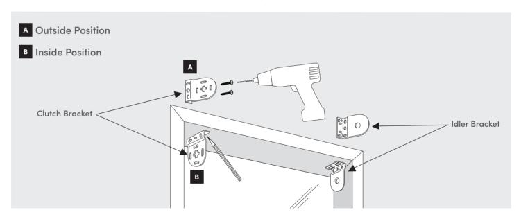
Inside / Outside Mount: Using a steel measuring tape, measure the distance from the outside edge of each bracket according to the ordered shade width. Mark the screw location on the mounting surface with a pencil, snap end caps onto brackets (if ordered).
