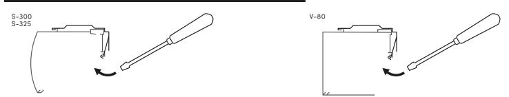
Insert a flat head screwdriver, between the bracket and cassette as shown. Gently pry the spring clip off the bracket of the cassette to unhook. The cassette should disengage from the bracket.
