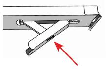
Push on the lever to extend the tensioner and secure your headrail.
