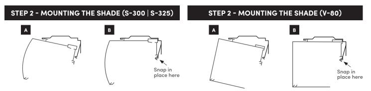
Hook the front of the cassette onto each bracket as shown in **(fig.A)**. Pivot the cassette back and snap into place **(fig.B)** on each bracket ensuring a tight and secure fit.
