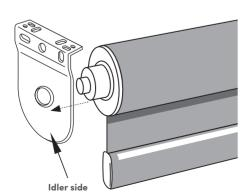
**B** - Ensure hook on the clutch side is pointing downward and securely fastens into the "+" shaped opening of the clutch bracket.
