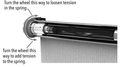
Reduce tension by turning the adjusting wheel upwards.
