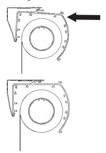
Step 3. Install the Bracket Covers - For Outside Mount Shades Only! Bracket covers slide onto the brackets as shown until they snap into position.
