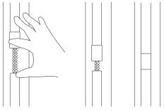
Slide the bottom section of the Chain Cover into the Connector that is pre-attached to the upper section
