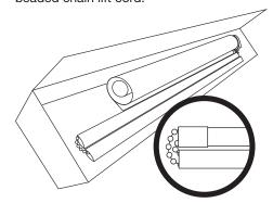
The cover for larger shades will be in two sections which are separated when the shade is packaged for shipment and thus must be joined together when the shade is installed. See complete instructions below:
