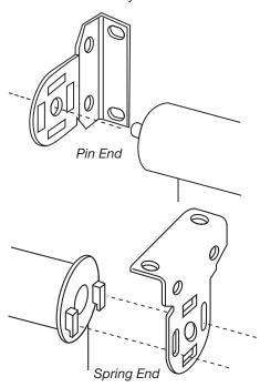
Step 2A. Cassette Installation (for shades with optional Cassette Valance) The shade is pre-mounted in the cassette. It can be removed to adjust tension, if necessary.
