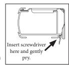
As you release the brackets, support the head rail to keep it from falling.
