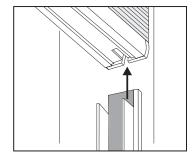
Front leg of track goes into slot in end cap and rail
