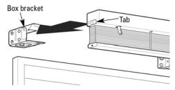
Lower the front gate of each box bracket and press until the locking tab clicks into place.
