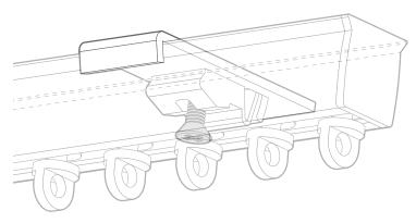
Clip the brackets onto the rail, spaced out as per page 1.
