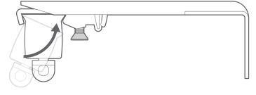
Rotate the headrail so that the back lip slots into the locking part of the bracket, then tighten the bracket screw to secure the rail in place.
