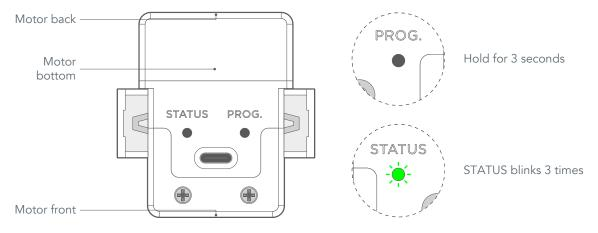
The motor is in its 'deep sleep' state when it is sent to you and will not operate until it is removed from this state. To do so, simply press and hold the PROG. button on the bottom of the motor for around 3 seconds, until the STATUS light blinks 3 times. The motor is now operational.
