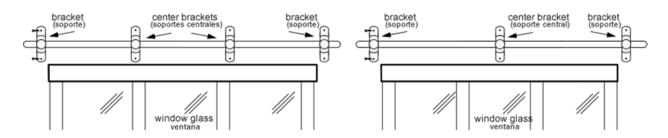
2. Mark screw locations using a pencil. It is recommended that the screws be driven directly into a wall stud. However, if this is not possible or practical, drywall anchors have been provided. Drill starter holes for the screws or screws & anchors.
