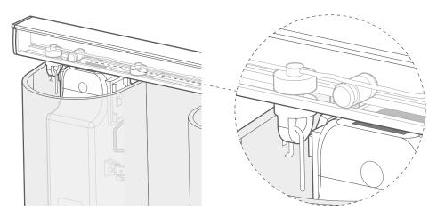
Lift the motor up behind the curtains and hook the runner that's still attached into the channel on the underside of the curtain rail.
