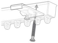
Drill a hole at each mark and insert rawl plugs. Then, hold the rail and brackets up and screw the brackets into place. Use a single screw for each bracket, through the rearmost screwhole.
