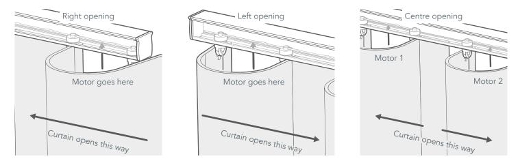
The motor will fit into the rail between the two outermost eyelets that the curtains are hooked onto, behind the curtains. For centre opening curtains you'll fit 2 motors, 1 behind each of the innermost eyelets. The motor should be fitted whilst the curtains are closed.
