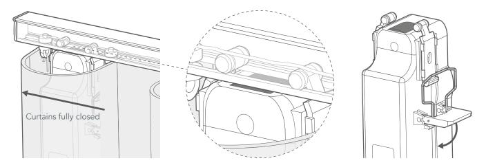
Take the runner you detached and hook it into place in the rail just as before, then clip it back into its mount on the side of the motor. Push the motor and curtain along the rail so that the curtains are in their fully closed position before locking the retaining clips on the sides of the motor.
