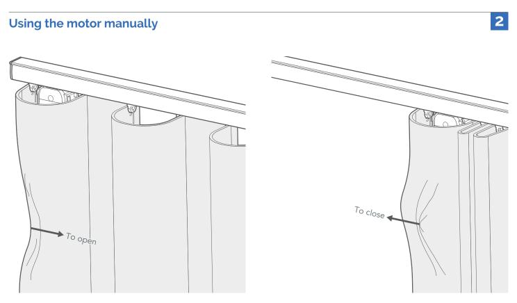
To open the curtains once the motor is installed, simply take the leading edge of the curtain and give it a sharp but gentle pull in the direction you want the curtain to open. The motor will detect the movement and engage, opening the curtain until fully open. To close the curtains, simply pull the leading edge of the curtain in the opposite direction.
