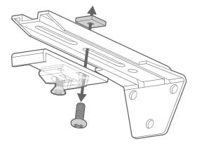
Detach the top fix section of the bracket from the L-shaped face fix section.
