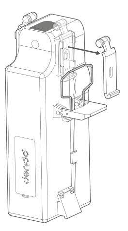
Start by unclipping one of the runners from the top of the motor. Lift the retaining clip then simply pull the runner free of its mounts on the side of the motor.
