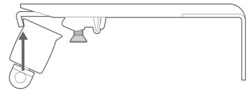
Locate the front lip of the curtain headrail into the front hook of the bracket.
