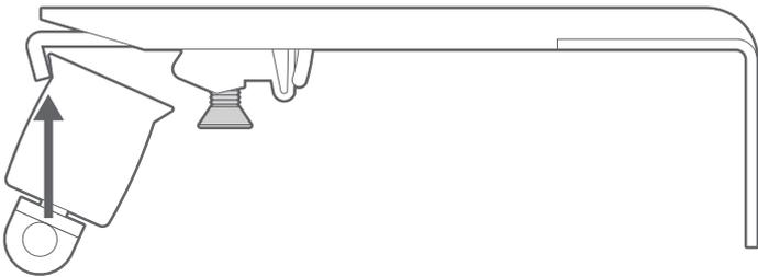
Locate the front lip of the curtain headrail into the front hook of the bracket.
