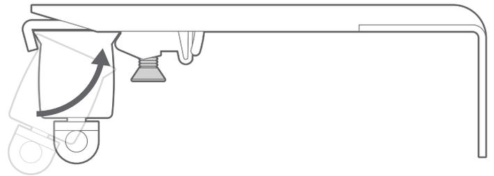
Rotate the headrail so that the back lip slots into the locking part of the bracket, then tighten the bracket screw to secure the rail in place.
