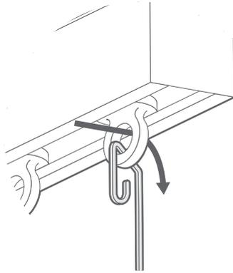
Insert the hooks into the plastic eyelets in the headrail.
