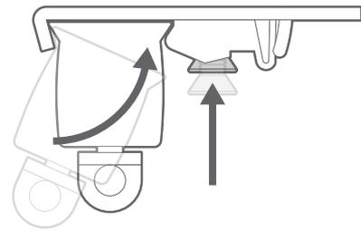
Rotate the headrail so that the back lip slots into the locking part of the bracket, then tighten the bracket screw to secure the rail in place.
