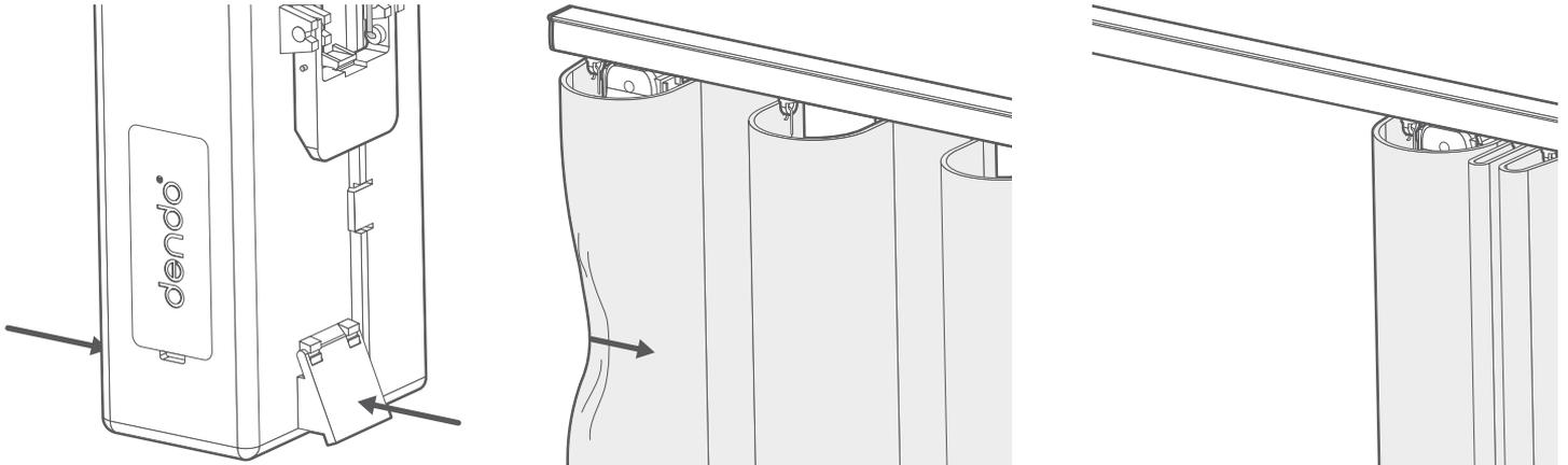
Whilst the curtains are in their closed position, reach up behind the fabric and press and hold both of the paddles on the sides of the motor at the same time, until the motor 'jogs' back and forth briefly. This has set the fully closed 'stop-point' position of the motor.
