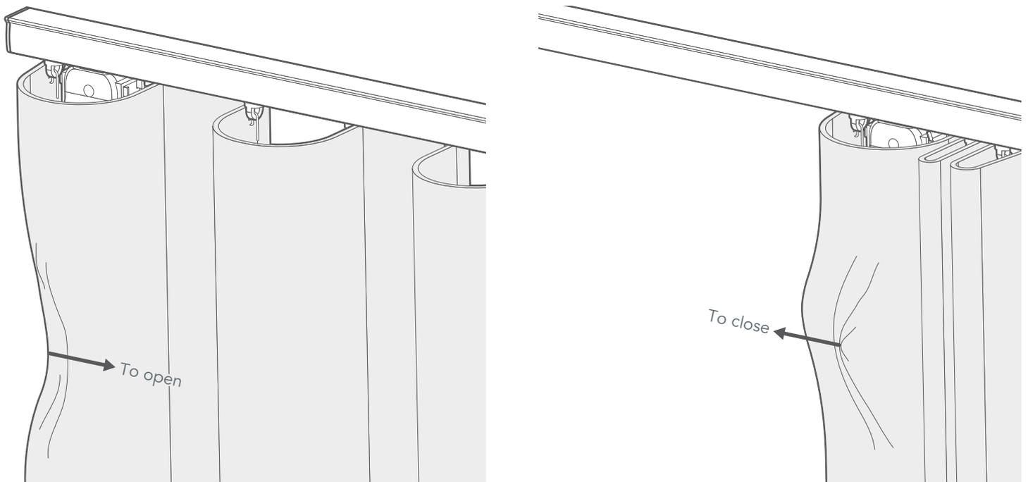
To open the curtains once the motor is installed, simply take the leading edge of the curtain and give it a sharp but gentle pull in the direction you want the curtain to open. The motor will detect the movement and engage, opening the curtain until fully open. To close the curtains, simply pull the leading edge of the curtain in the opposite direction.
