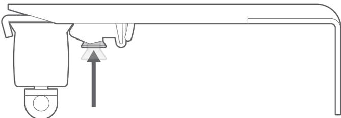
Tighten the locking screw in the bracket to lock the rail in place.
