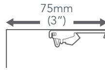
If you are using top-fix brackets, the front edge of the bracket must be at least 75mm (3") away from the facing surface behind the rail. This will ensure that the waves in the fabric do not brush against the wall or window behind.
