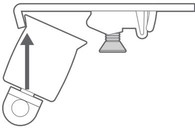
To do so, locate the front lip of the curtain headrail into the front hook of the bracket.
