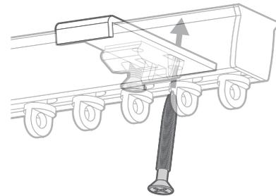
Drill a hole at each mark and insert rawl plugs. Then, hold the rail and brackets up and screw the brackets into place. Use a single screw for each bracket, through the rear-most screw hole.
