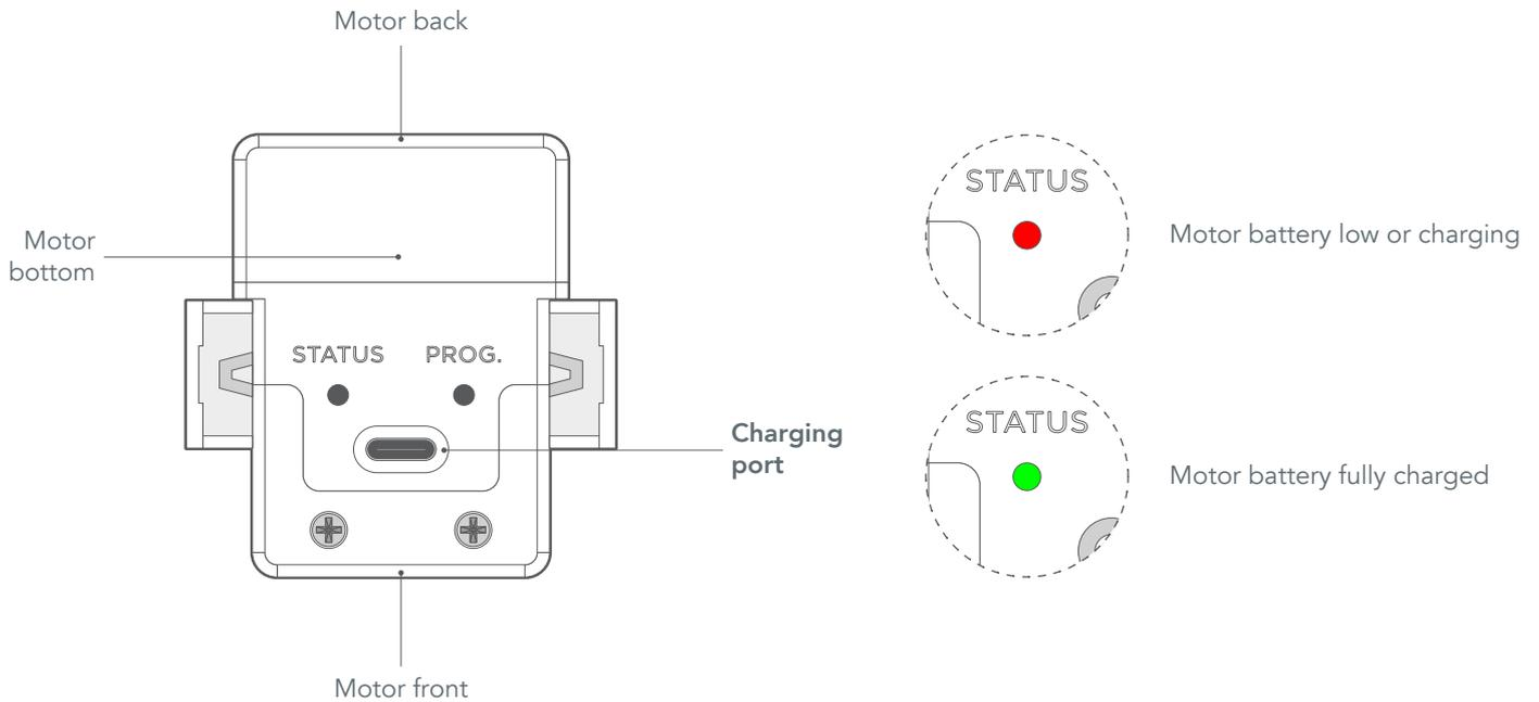
The motor has a USB-C charging port on the bottom. To charge the motor's battery, simply plug the charging cable into the charging port. A full charge typically takes around 8 hours if the battery is fully depleted. Whilst charging, the STATUS light on the bottom of the motor will glow red, then change to green when fully charged.
