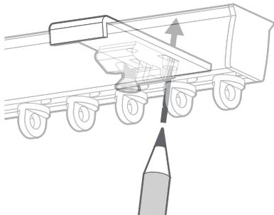
Next, hold the rail up to the fitting surface and mark out the screw holes with a pencil.
