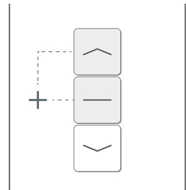
Hold the OPEN and STOP buttons until the motor 'jogs'. The motor is now deleted from that channel.
