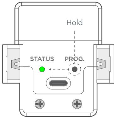
On the bottom of the motor, press and hold the PROG. button until the STATUS light turns green.
