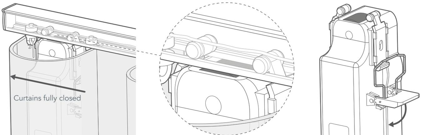
Take the runner you detached and hook it into place in the rail just as before, then clip it back into its mount on the side of the motor. Push the motor and curtain along the rail so that the curtains are in their fully closed position before locking the retaining clips on the sides of the motor.
