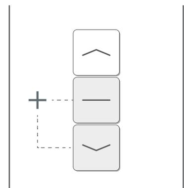
Hold the CLOSE and STOP buttons until the motor 'jogs'. The motor is now deleted from all channels.
