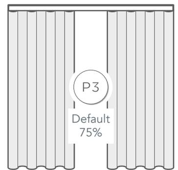
By default, pressing P1 will move the curtains to 25% closed, P2 to 50% closed and P3 to 75% closed, but these positions can be changed if preferred.
