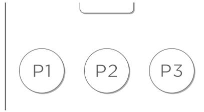
The motor can be set to automatically move the curtains to other positions besides fully open or closed. Default 'intermediate stop-points' are paired to the P1, P2 and P3 buttons on the remote control automatically.
