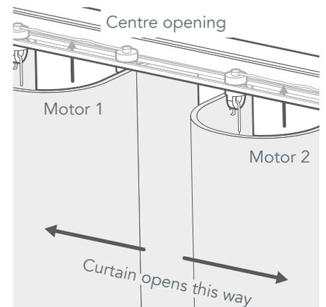
The motor will fit into the rail between the two outermost eyelets that the curtains are hooked onto, behind the curtains. For centre opening curtains you'll fit 2 motors, 1 behind each of the innermost eyelets. **The motor should be fitted whilst the curtains are closed.**
