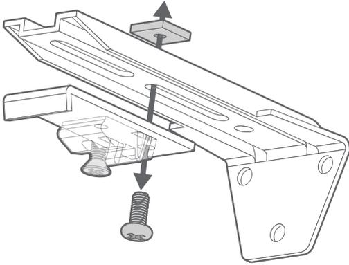
Detach the top fix section of the bracket from the L-shaped face fix section.
