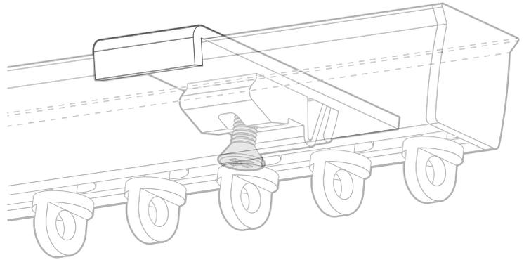
Clip the brackets onto the rail, spaced out as per page 1.
