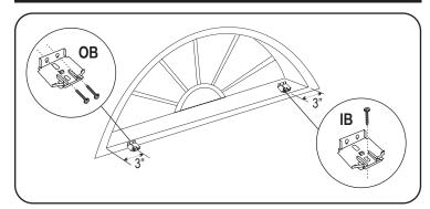
Mount end brackets 3" from each side and space any remaining brackets evenly. Make sure that all brackets are aligned and level.
