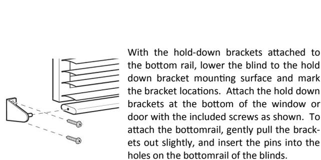
With the hold-down brackets attached to the bottom rail, lower the blind to the hold down bracket mounting surface and mark the bracket locations. Attach the hold down brackets at the bottom of the window or door with the included screws as shown. To attach the bottomrail, gently pull the brackets out slightly, and insert the pins into the holes on the bottomrail of the blinds.
