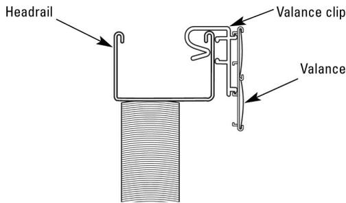
**Outside Mount Valances:** For aluminum blinds ordered as outside mount, the aluminum slats used for the valance, will be made wider than the headrail. Attach the slats to the plastic valance clips, and then bend both the left and right sides of the valance so that the aluminum valance slats cover the box installation brackets.
