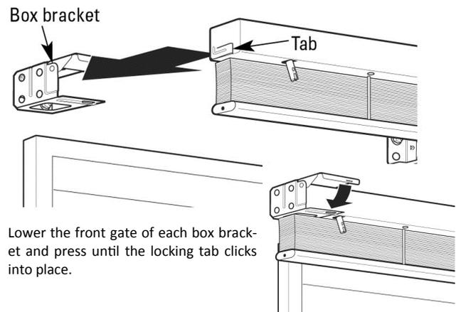
Lower the front gate of each box bracket and press until the locking tab clicks into place.
